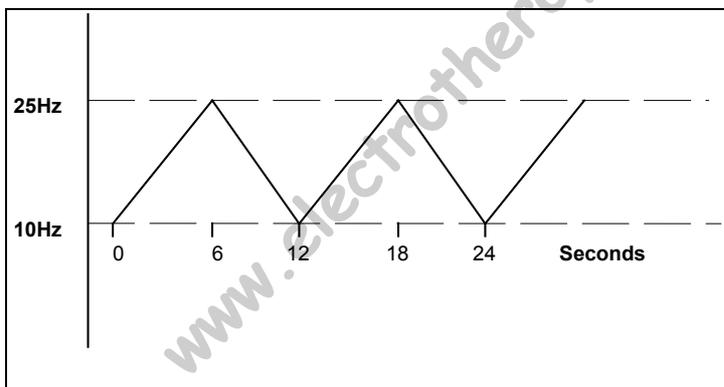
The mode of delivery of the selected sweep varies with machines. The most common application is the 6 second rise and fall between the pre-set frequencies. For example, if a 10 - 25Hz range has been selected, the machine will deliver a changing frequency, starting at 10Hz, rising to 25Hz over a 6 second period. Once this upper limit has been
